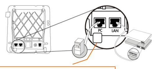
Plug the Ethernet cable into the back of the base station.
