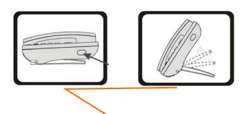
Press and hole the button of right side to change the stand mount angle.
