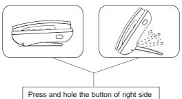
Press and hole the button of right side to change the stand mount angle.
