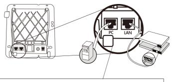
Plug the Ethernet cable into the back of the base station. Plug the other end of the Ethernet cable into your already prepared network connection.
