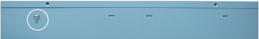
IDL-2402 grounding screw on the rear panel
