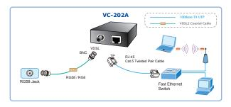
Figure 3-7: Connecting Multiple PCs to an Ethernet LAN
