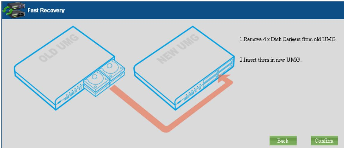
If the following screen appears, it means the fast recovery has completed successfully. Otherwise, check the devices. After the rebuilding, the UMG-2000 / UMG-2200 will reboot automatically. Then the new UMG can serve normally.
