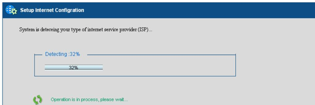
The ISP type will be detected and the result will be presented as follows. If “Network Cable Disconnected” is detected, please recheck the physical connection and repeat the action as shown in Section “WAN Connection”. There could be more than one ISP type recognized, so choose the most suitable type from the list and then click the button “Next” to continue.
