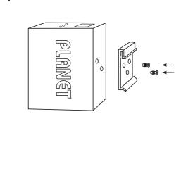
Step 3: Check the DIN-Rail is tightly on the track.
