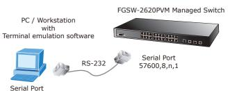
A terminal program is required to make the software connection to the PoE Switch / FGSW-2624SF. Windows' **Hyper Terminal** program may be a good choice. The Hyper Terminal can be accessed from the **Start** menu.
