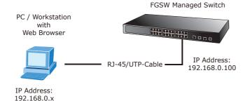
The following shows how to startup the **Web Management** of the **Managed Switch**, please note the Managed Switch is configured through an Ethernet connection, make sure the manager PC must be set on the same **IP subnet** address.
