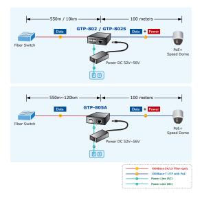
For the places where are hard to find the power inlet, the GTP-80X provide the easiest way to power your Ethernet devices such as PLANET IEEE 802.3at / 802.3af Power over Ethernet Splitter (POE-151S / 152S / 161S) with Internet Camera or PoE Wireless Access Point installed in the wild rang place.
