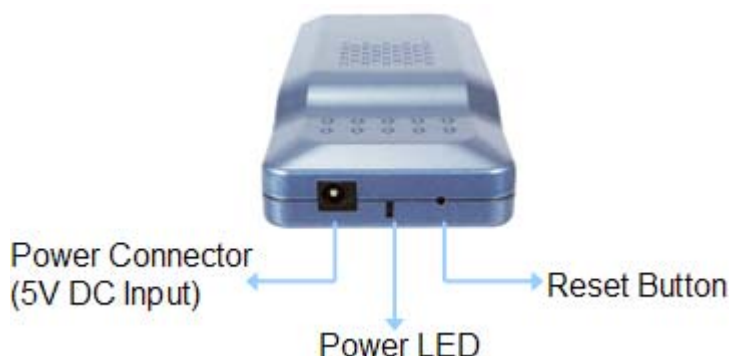
Figure 2-1 The WPG-130N Front Panel
