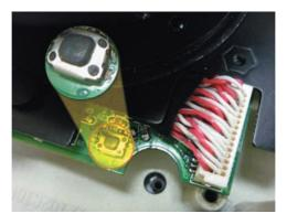
2. Connect power to the camera again, and do not release the button during the system booting.
