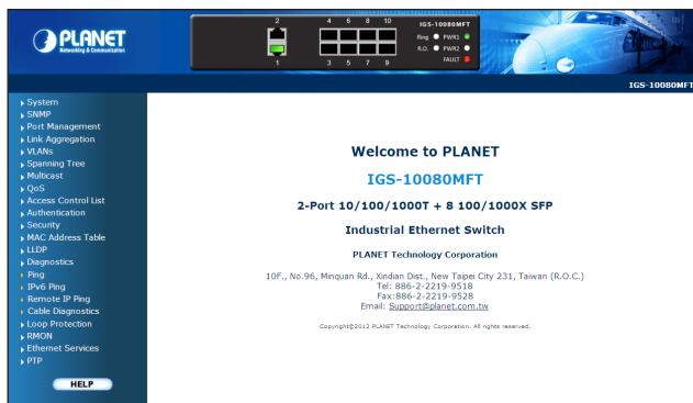
Figure 7-3 Web Main Screen of Industrial Managed Switch
