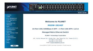
Figure 7-3: Web Main Screen of the Managed Switch
