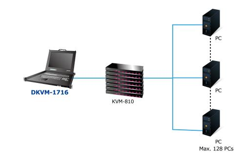
The combo-free KVM is connected to any PC or server directly without concern of keyboard / mouse interface compatibility.
