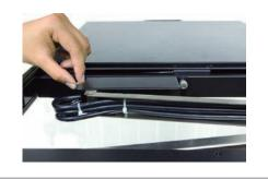
STEP 4: Please fix KVM module with the rack mount bracket kit
