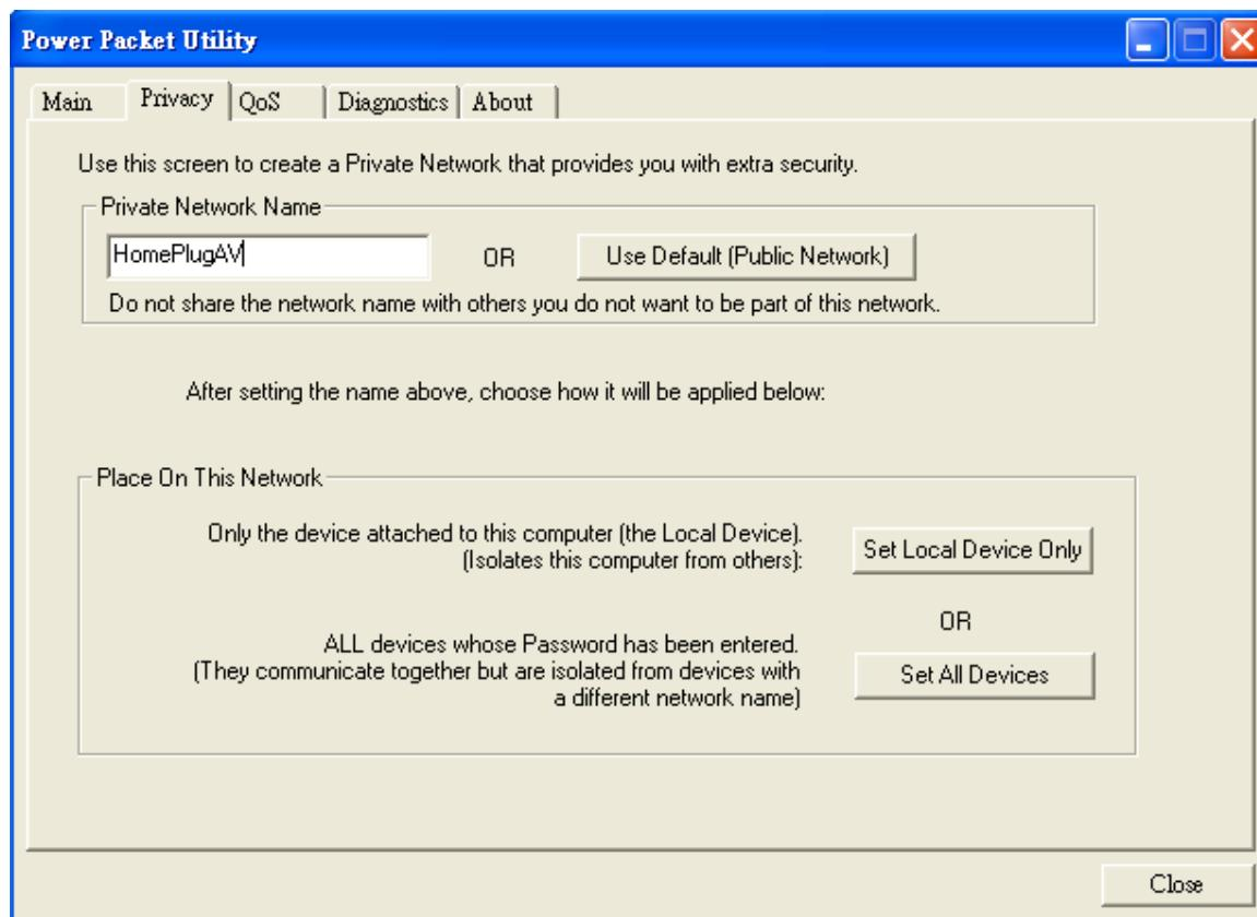
The **Privacy** tab will allow you to change the **Network Password** to the unit that is currently connected to this computer. This network password encrypts all data that is sent from this unit using 128-bit data encryption standard (AES).
