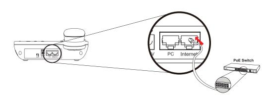
NOTE: Only internet port of the VIP-256PT support 802.3af power injection, use of any non-standard POE injector could damage the device.
