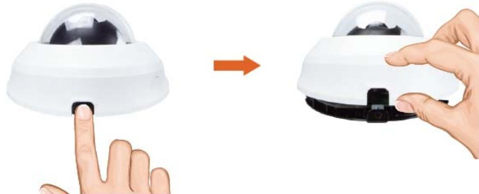
Press the button to release the case.
