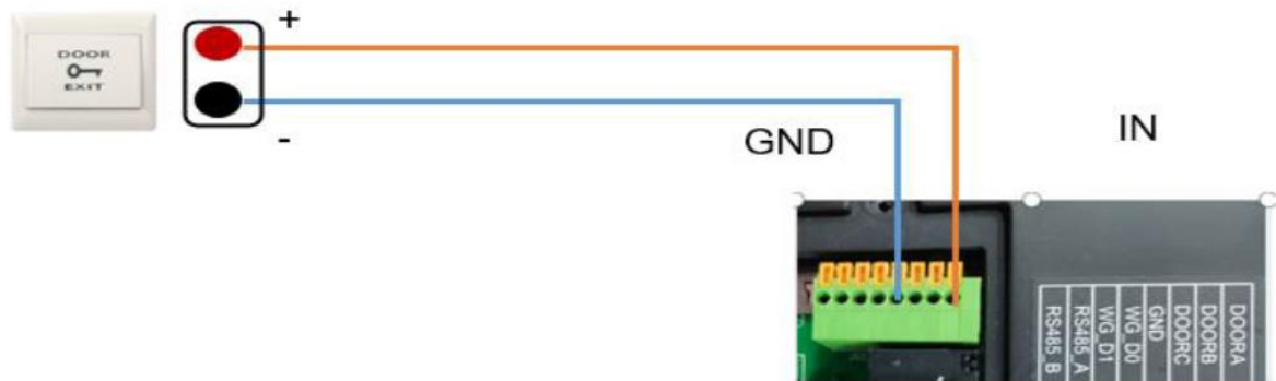
Figure 3-5-1 Connect a push-to-exit button to the door phone
